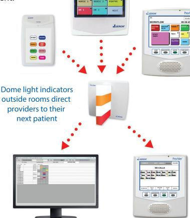
Each room's status is visible from wall-mounted displays and networked computers
